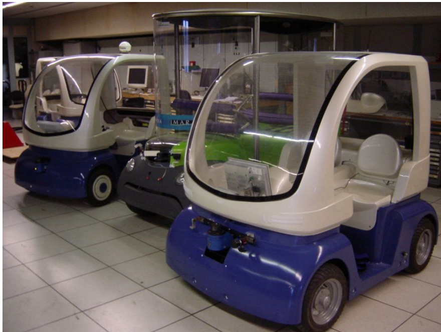
Figure 1.1: Different types of cybercars: two CyCabs and one AGV. Reproduced with permission from Imara, courtesy of Rodrigo BENENSON.
