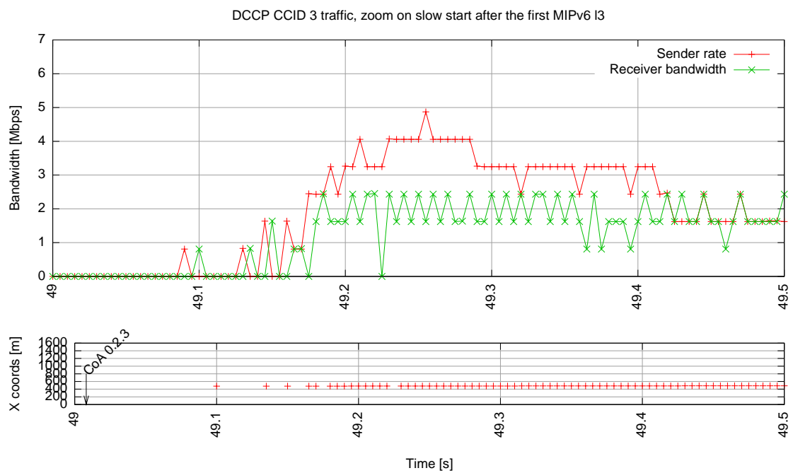
Figure 5.9: A very close zoom of the end of the first DCCP handover with 3 base stations. One can see the initial slow start ( 49.08 \leq t \leq 49.17 ) due to the wrong assumption that the previous packet losses were due to a congested network. The algorithm then overshoots the maximum available bandwidth ( t = 49.19 ) and subsequently adjusts its rate ( t \geq 49.4 ).
