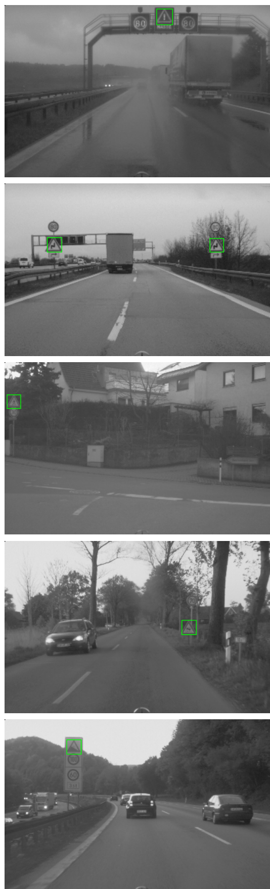
Fig. 7. Examples of detections using the 576 value HOG detector. Our dataset contains images taken in urban, country road and highway environments under different illumination and weather conditions.
