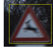
Fig. 5. Tight bounding box of the traffic sign used for computing HOG 4 feature
