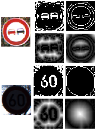
Fig. 2. Comparison of Distance Transforms (DT) using bottom hat thresholding and Canny edge detection. Left: original image, center: bottom hat threshold result and corresponding DT, right: Canny edge detection and corresponding DT
