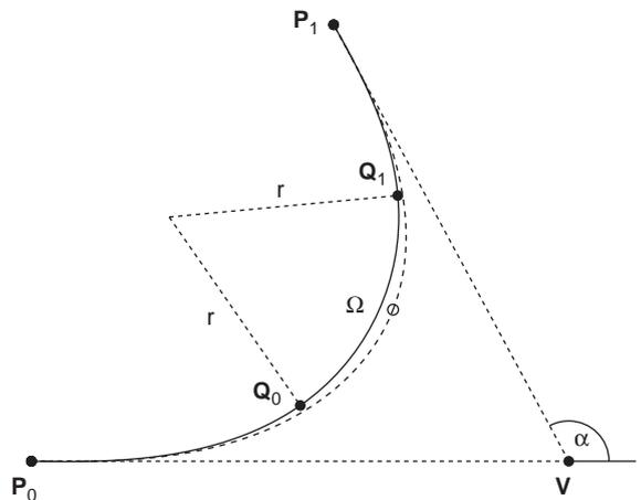
Fig. 6. Unsymmetric circular arc insertion.
