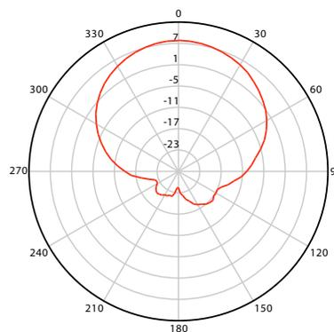
Azimuth Radiation Pattern (Normalized to 0dbi.)
